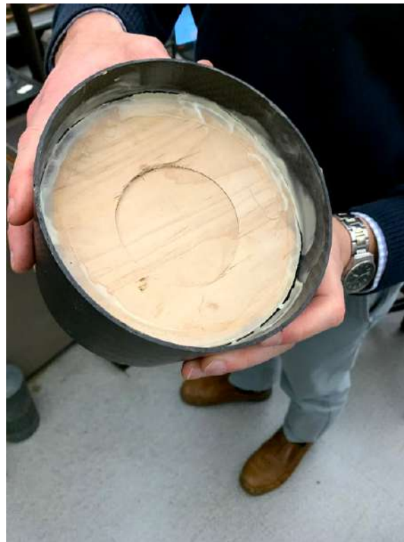
Figure 22: Plywood Failed Bulkhead
